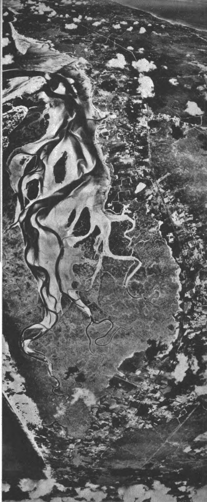
75-mile-long Cape Cod peninsula is filmed in a single picture made with new Air Force pendulum camera that can take a picture, horizon to horizon in a two-second swing.
